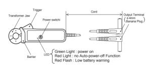
One press of the Power Switch powers on the instrument and the green LED lights up. Another press of the Power Switch powers off the instrument. The instrument is automatically powered off in about 20 min after the last switch operation. (Auto-power-off Function)
